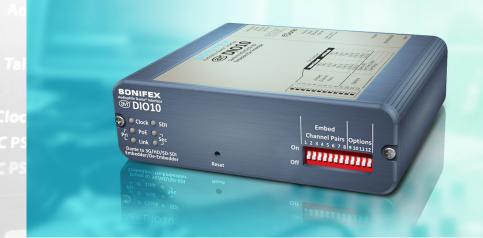
The unique **AVN-DIO10** is used for simultaneously embedding and de-embedding SDI signals to and from the Dante® AoIP audio network. It takes an SDI feed, de-embeds the 16 audio channels and places them on channels 1-16 of the Dante network, mapped using Dante Controller. It simultaneously takes the 16 input channels mapped to the device on Dante Controller and re-embeds them onto the SDI output.
